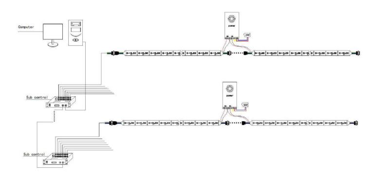
**3.Main controller + sub controller(Big project)** Recommended controller:Main controller: XB-Z2/MR-BF12B, Sub controller :T-780K/MR-218DW
