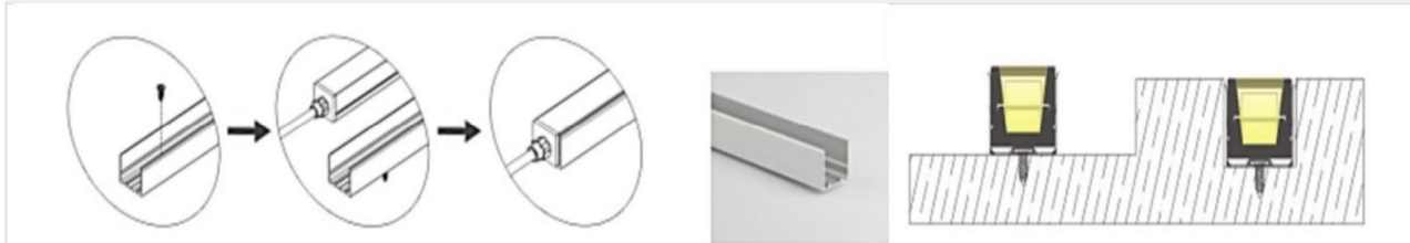
Aluminum Channel and Flexible Wall Washer Installation Schematic
